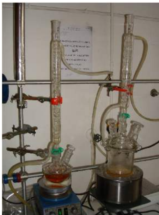
Figure 2. The experimental setup used for the discovery of the impact of light on aqueous solutions produced by thermally processing carrot ( Daucus carota L.) roots in water.
