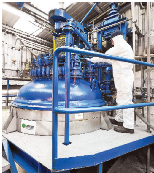
A technician works on a multipurpose batch reactor at Almac's Arran Chemical facility, where the company works on immobilizing the enzyme on polymer beads for Alcresta Therapeutics.
